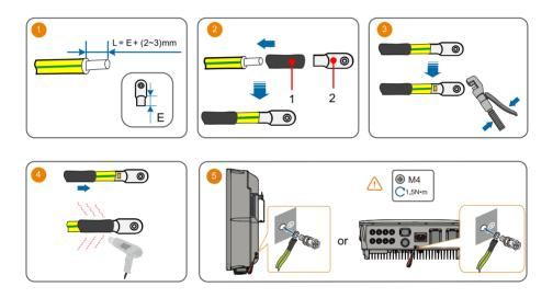
• The cable specification must comply with local regulations (if available). Otherwise, keep it consistent with the PE wire in the AC cable.
