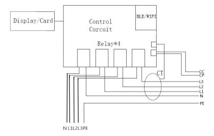
Schematic representation of the wiring
