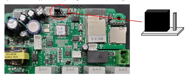
In order to use the RFID cards to activate the charging process, the jumper marked in the above image must be in the position shown. If the AXIbox was previously in Plug & Play mode, the jumper must be moved back to the position shown above to switch to RFID mode.
